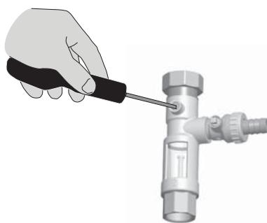
**Note:** In high efficiency hydraulic units, the pump modulates the flow based on the temperature difference between the solar collectors and the accumulator, therefore manual adjustment is not required. The manual flow regulator is used if the pump needs to be isolated.
