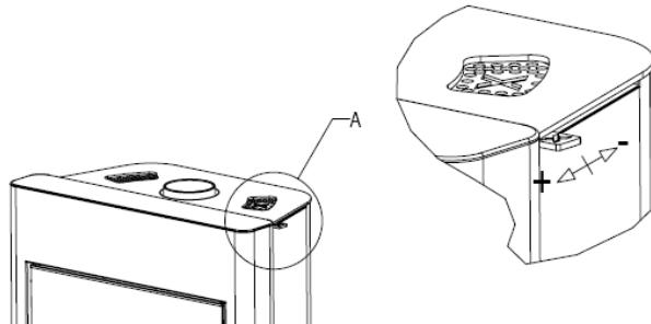
Our hint: while the fire still burns let the convection air outlets open; close them after the fire has burnt down in order to reach a steady heat emission.
